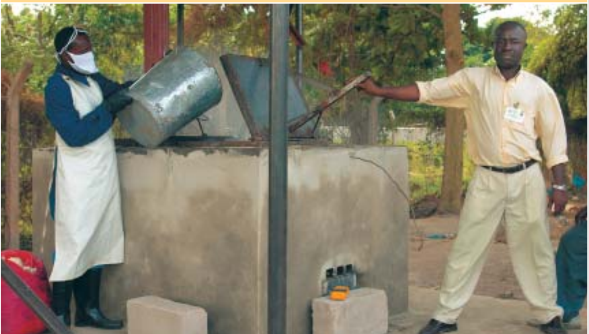
Low cost, locally built incinerators in Africa
